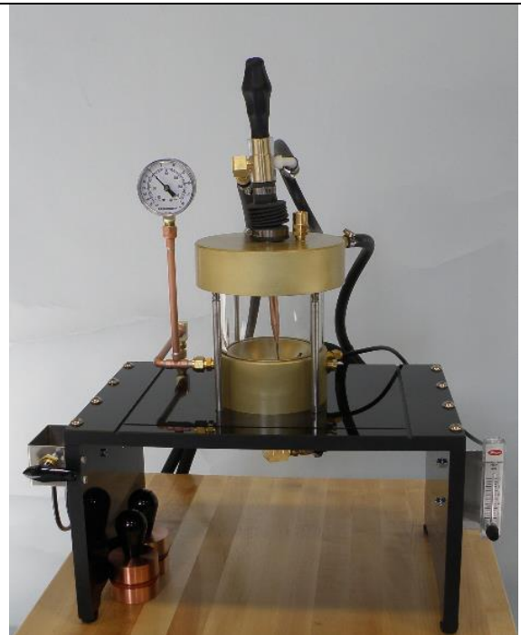
Basic unit with gas and vacuum system. Welding glasses and shield have been removed for clarity.
